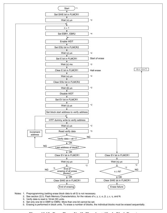
Figure 19.13 Erase/Erase-Verify Flowchart (Single-Block Erase)
