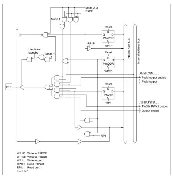
Figure C.1 Port 1 Block Diagram (Pins P10 and P11)
