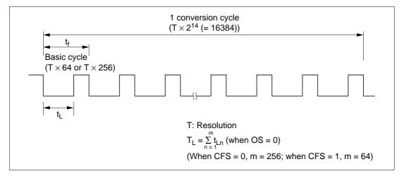
Figure 10.3 PWM D/A Operation
