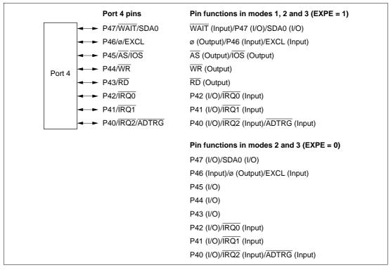
Figure 8.12 Port 4 Pin Functions
