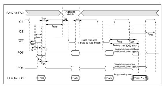
Figure 19.20 Auto-Program Mode Timing Waveforms
