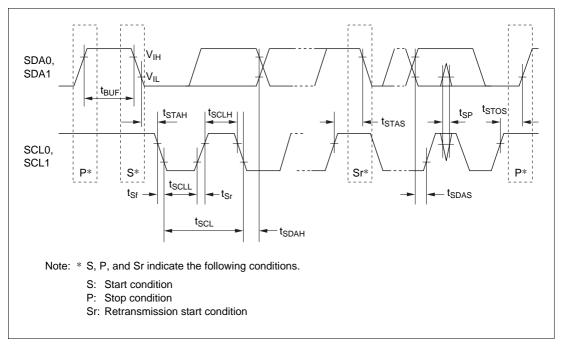
Figure 22.24 I<sup>2</sup>C Bus Interface Input/Output Timing (Option)
