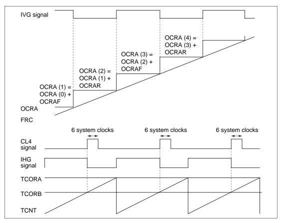
Figure 13.8 IVG Signal/IHG Signal/CL4 Signal Timing Chart
