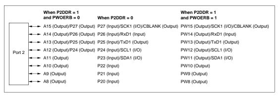
Figure 8.7 Port 2 Pin Functions (Modes 2 and 3 (EXPE = 1))
