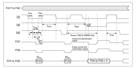
Figure 19.21 Auto-Erase Mode Timing Waveforms
