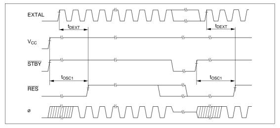
Figure 22.5 Oscillation Settling Timing
