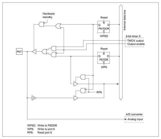
Figure C.22 Port 6 Block Diagram (Pin P67)
