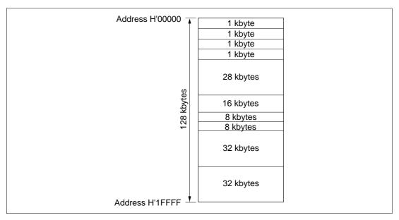
Figure 19.6 Flash Memory Block Configuration
