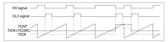
Figure 13.4 Timing Chart for Clamp Waveform Generation (CL3 Signal)
