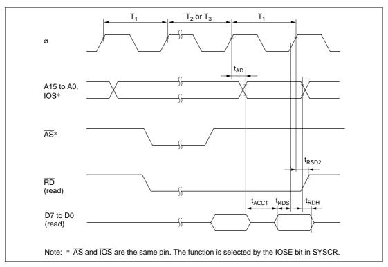
Figure 22.13 Burst ROM Access Timing (One-State Access)
