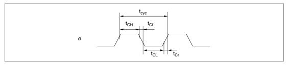
Figure 22.4 System Clock Timing
