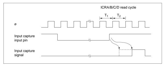
Figure 11.8 Input Capture Signal Timing (Input Capture Input when ICRA/B/C/D is Read)
