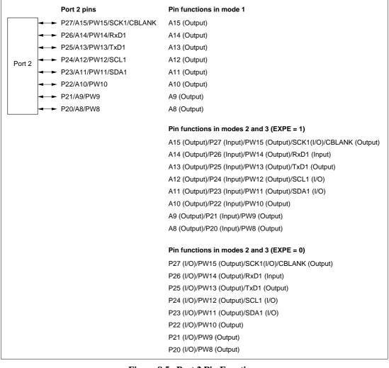
Figure 8.5 Port 2 Pin Functions
