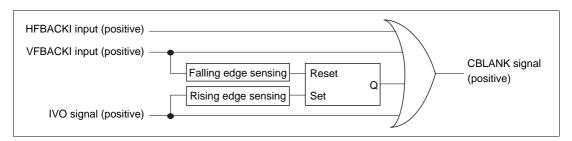
Figure 13.9 CBLANK Output Waveform Generation
