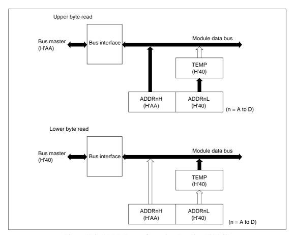
Figure 17.2 ADDR Access Operation (Reading H'AA40)
