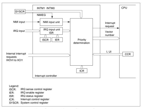
Figure 5.1 Block Diagram of Interrupt Controller
