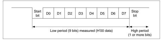
Figure 19.9 RxD0 Input Signal when Using Automatic SCI Bit Rate Adjustment
