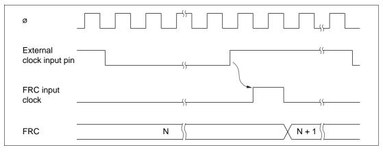
Figure 11.4 Increment Timing with External Clock Source
