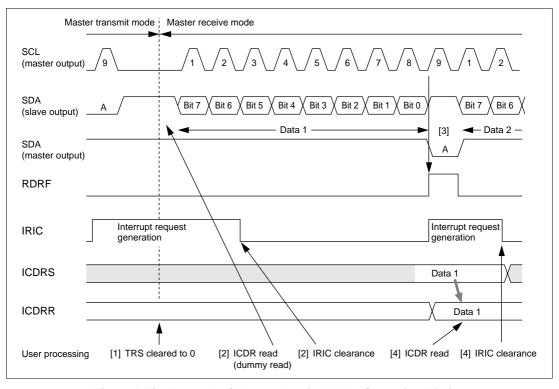
Figure 16.8 Example of Master Receive Mode Operation Timing (MLS = WAIT = ACKB = 0)
