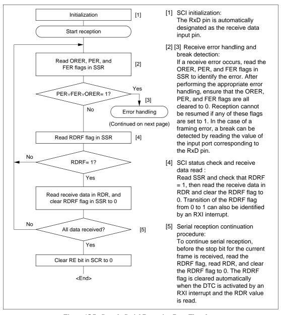
Figure 15.7 Sample Serial Reception Data Flowchart
