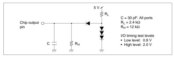
Figure 22.3 Output Load Circuit
