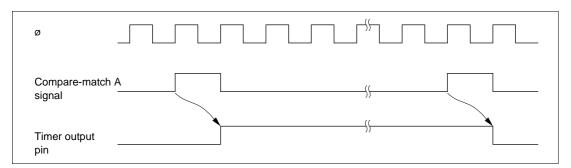
Figure 12.5 Timing of Timer Output
