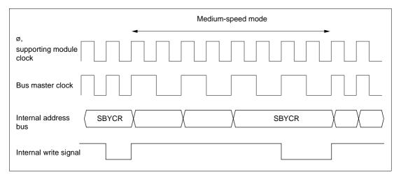
Figure 21.2 Medium-Speed Mode Transition and Clearance Timing
