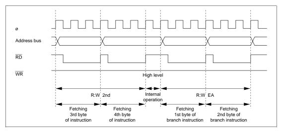
Figure A.1 Address Bus, RD, WR Timing (8-Bit Bus, Three-State Access, No Wait States)
