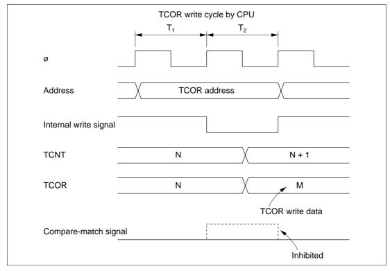
Figure 12.12 Contention between TCOR Write and Compare-Match
