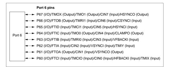
Figure 8.14 Port 6 Pin Functions
