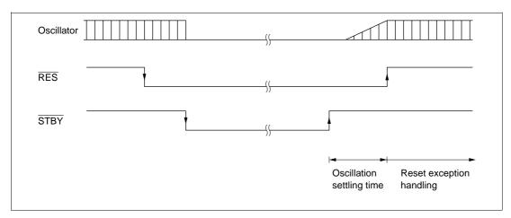
Figure 21.4 Hardware Standby Mode Timing
