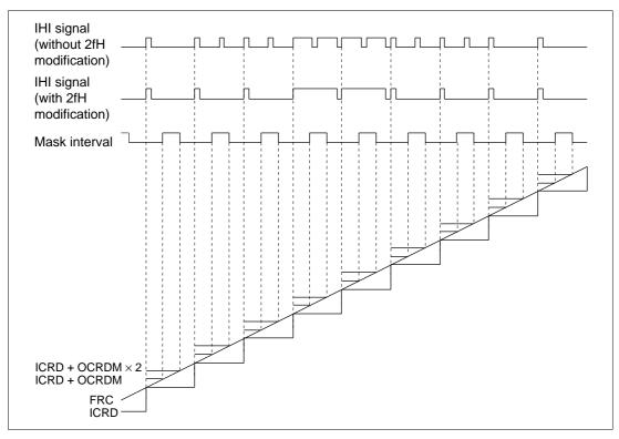
Figure 13.6 2fH Modification Timing Chart
