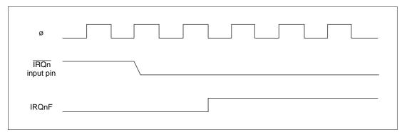
Figure 5.3 Timing of IRQnF Setting
