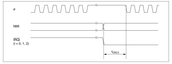
Figure 22.6 Oscillation Setting Timing (Exiting Software Standby Mode)
