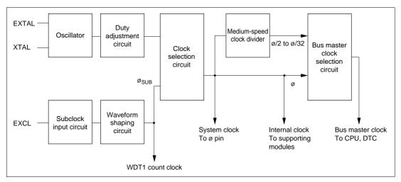
Figure 20.1 Block Diagram of Clock Pulse Generator
