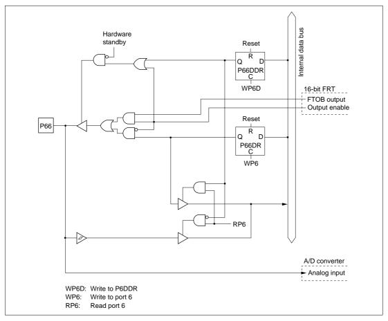
Figure C.21 Port 6 Block Diagram (Pin P66)
