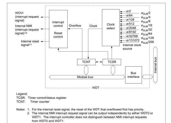
Figure 14.1 (b) Block Diagram of WDT1
