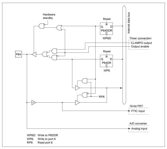
Figure C.20 Port 6 Block Diagram (Pin P64)
