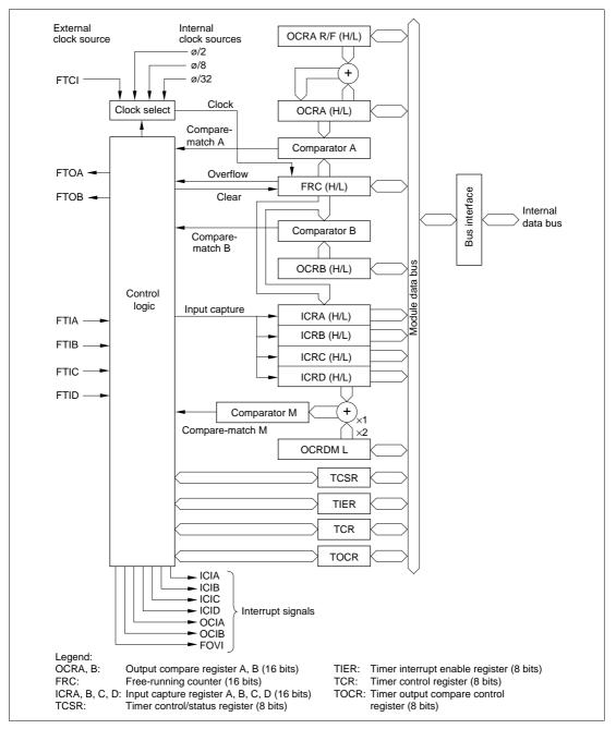
Figure 11.1 Block Diagram of 16-Bit Free-Running Timer
