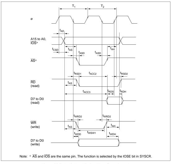
Figure 22.9 Basic Bus Timing (Two-State Access)
