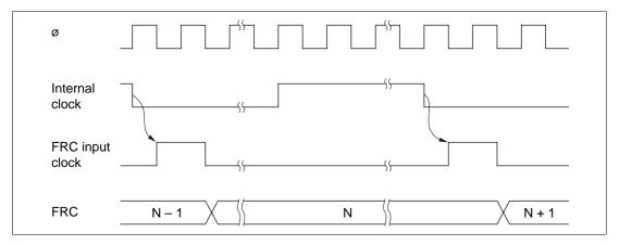
Figure 11.3 Increment Timing with Internal Clock Source
