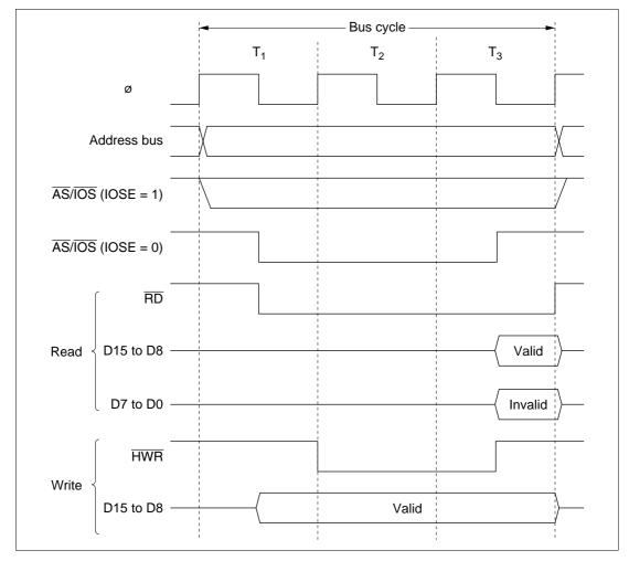
Figure 6.6 Bus Timing for 8-Bit 3-State Access Space
