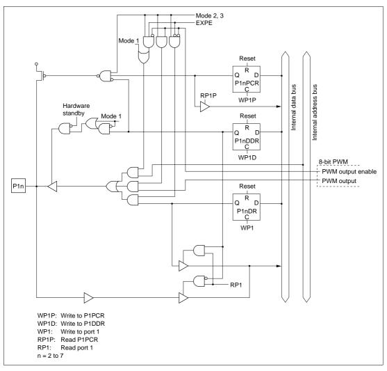
Figure C.2 Port 1 Block Diagram (Pins P12 to P17)
