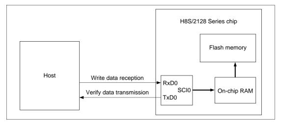
Figure 19.7 System Configuration in Boot Mode
