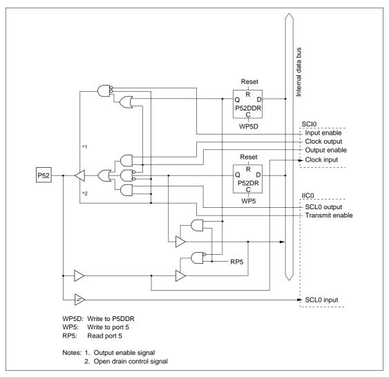
Figure C.17 Port 5 Block Diagram (Pin P52)
