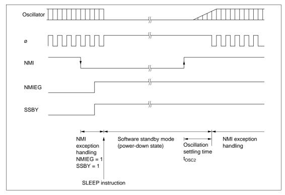
Figure 21.3 Software Standby Mode Application Example
