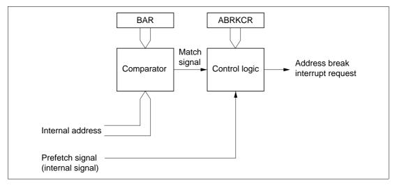
Figure 5.4 Block Diagram of Address Break Function
