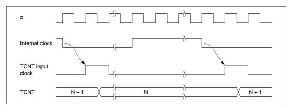
Figure 12.2 Count Timing for Internal Clock Input
