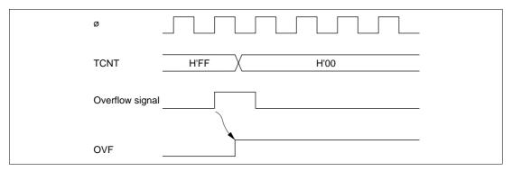
Figure 12.8 Timing of OVF Setting
