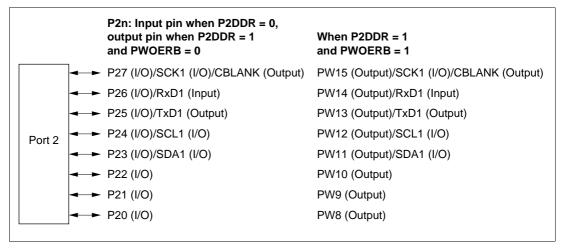
Figure 8.8 Port 2 Pin Functions (Modes 2 and 3 (EXPE = 0))
