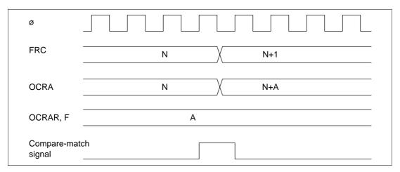
Figure 11.14 OCRA Automatic Addition Timing
