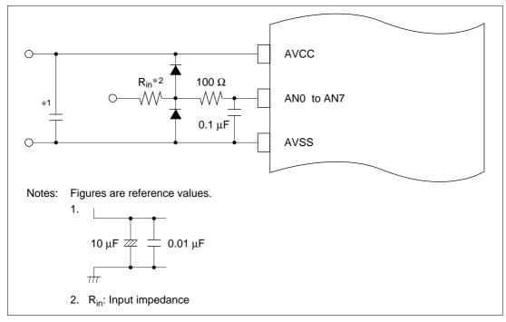
Figure 17.7 Example of Analog Input Protection Circuit
