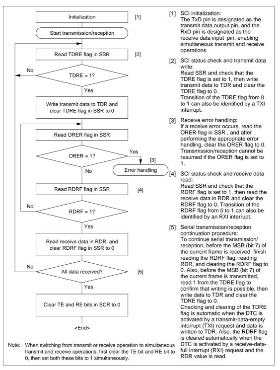
Figure 15.20 Sample Flowchart of Simultaneous Serial Transmit and Receive Operations
