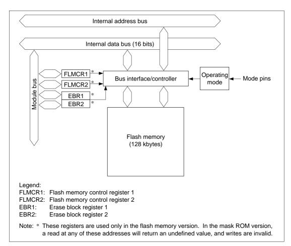
Figure 19.2 Block Diagram of Flash Memory
