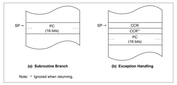
Figure 2.3 Stack Structure in Normal Mode
