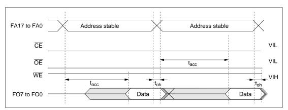
Figure 19.18 Timing Waveforms for  $\overline{\text{CE}}/\overline{\text{OE}}$  Enable State Read
