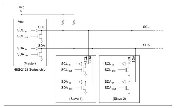
Figure 16.2 I<sup>2</sup>C Bus Interface Connections (Example: H8S/2128 Series Chip as Master)
