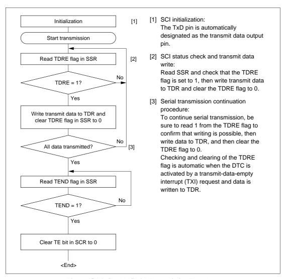
Figure 15.16 Sample Serial Transmission Flowchart
