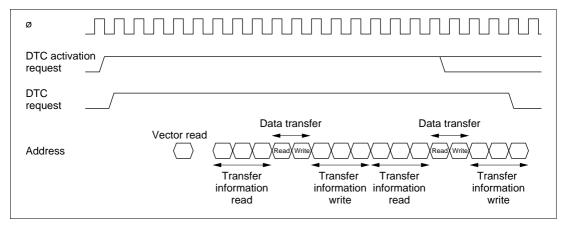
Figure 7.12 DTC Operation Timing (Chain Transfer)
