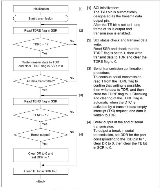
Figure 15.5 Sample Serial Transmission Flowchart
