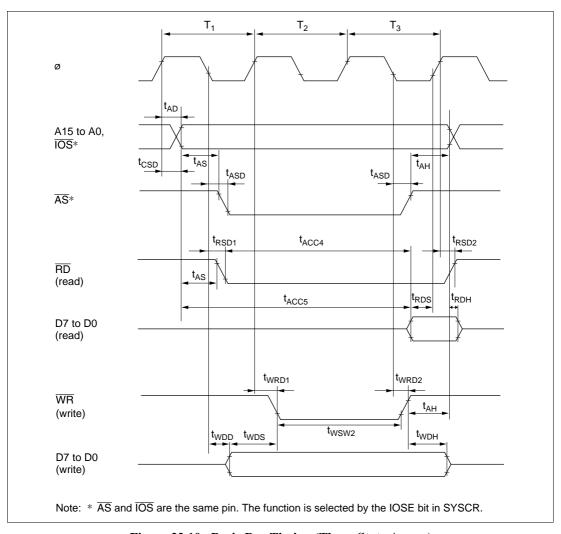
$Figure\ 22.10\quad Basic\ Bus\ Timing\ (Three-State\ Access)$
