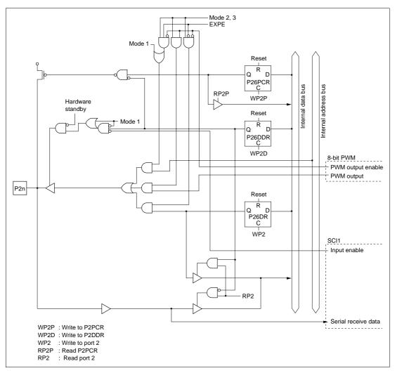
Figure C.7 Port 2 Block Diagram (Pin P26)
