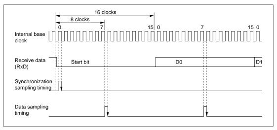
Figure 15.21 Receive Data Sampling Timing in Asynchronous Mode
