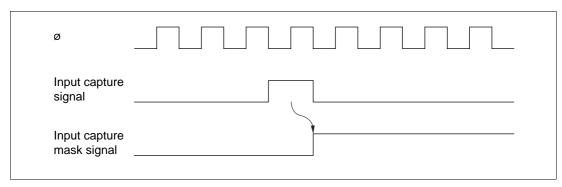
Figure 11.15 Input Capture Mask Signal Setting Timing
