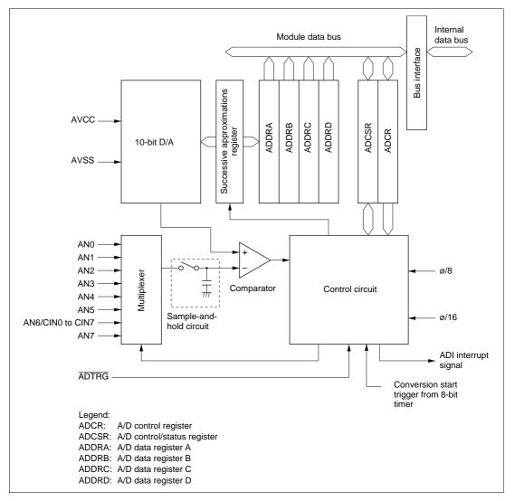
Figure 17.1 Block Diagram of A/D Converter
