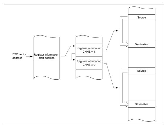
Figure 7.9 Memory Mapping in Chain Transfer
