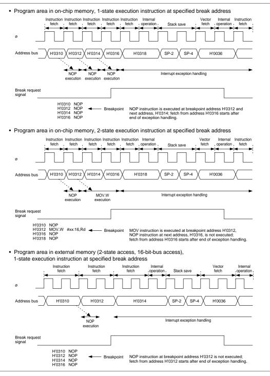
Figure 5.5 Examples of Address Break Timing
