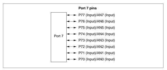
**Figure 8.15 Port 7 Pin Functions**
