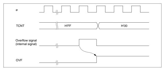
Figure 14.5 Timing of OVF Setting
