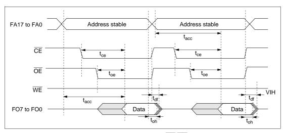
Figure 19.19 Timing Waveforms for  $\overline{\text{CE}}/\overline{\text{OE}}$  Clocked Read
