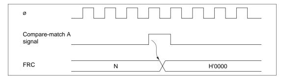
Figure 11.6 Clearing of FRC by Compare-Match A
