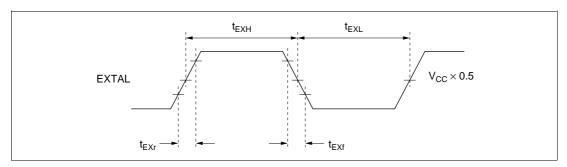
Figure 20.6 External Clock Input Timing
