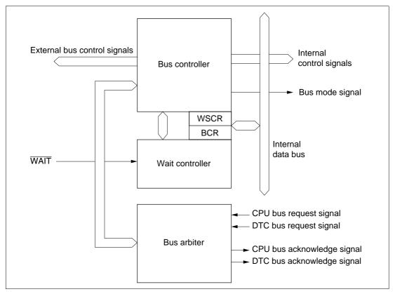
Figure 6.1 Block Diagram of Bus Controller
