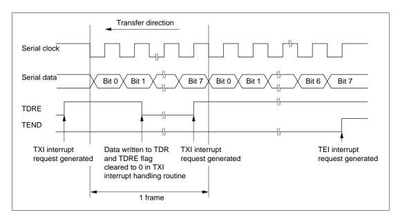
Figure 15.17 Example of SCI Operation in Transmission
