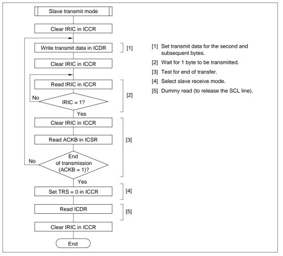
Figure 16.17 Flowchart for Slave Transmit Mode (Example)
