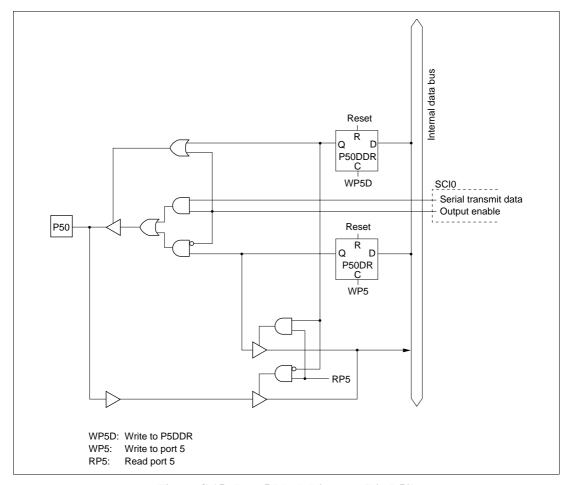
Figure C.15 Port 5 Block Diagram (Pin P50)
