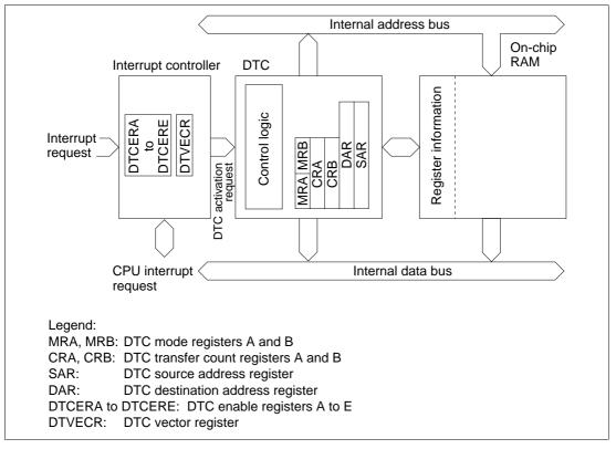
Figure 7.1 Block Diagram of DTC
