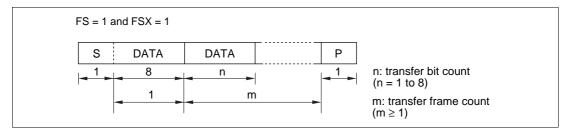
Figure 16.4 I<sup>2</sup>C Bus Data Format (Serial Format)
