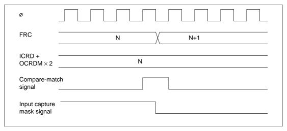
Figure 11.16 Input Capture Mask Signal Clearing Timing
