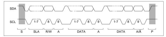
Figure 16.5 I<sup>2</sup>C Bus Timing
