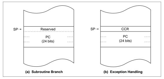
Figure 2.5 Stack Structure in Advanced Mode
