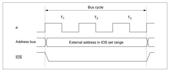
Figure 6.2 **IOS** Signal Output Timing
