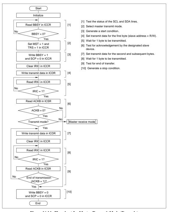
Figure 16.14 Flowchart for Master Transmit Mode (Example)
