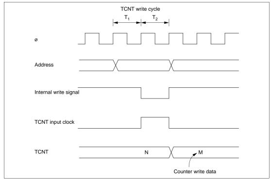
Figure 14.6 Contention between TCNT Write and Increment
