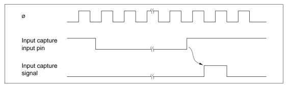
Figure 11.7 Input Capture Signal Timing (Usual Case)
