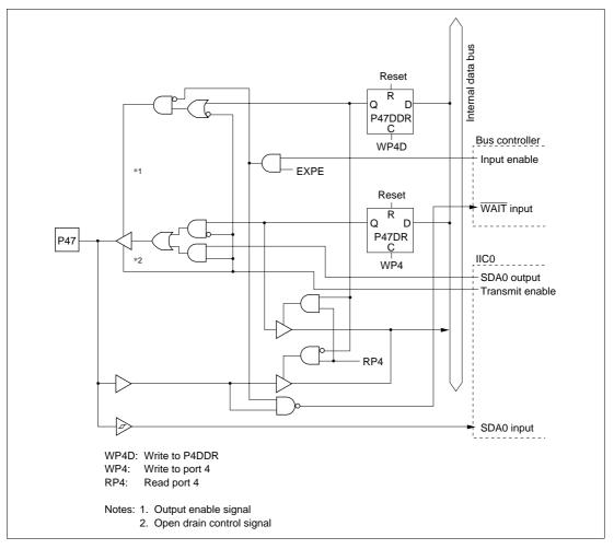
Figure C.14 Port 4 Block Diagram (Pin P47)
