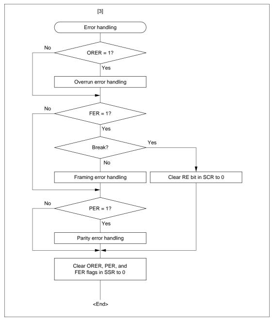
Figure 15.7 Sample Serial Reception Data Flowchart (cont)
