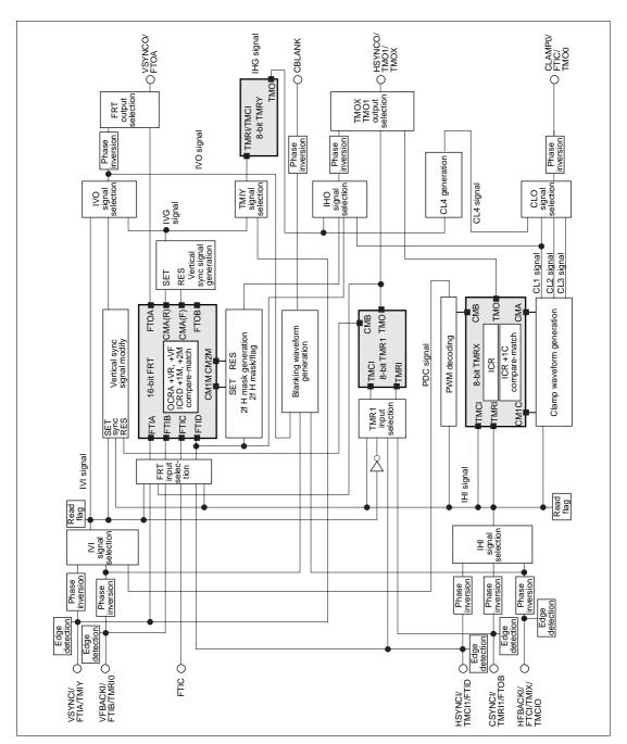
Figure 13.1 Block Diagram of Timer Connection Facility
