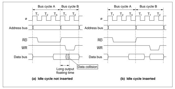
Figure 6.9 Example of Idle Cycle Operation
