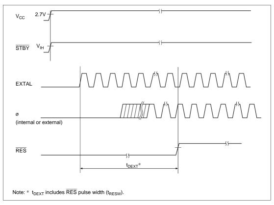
Figure 20.7 External Clock Output Settling Delay Timing
