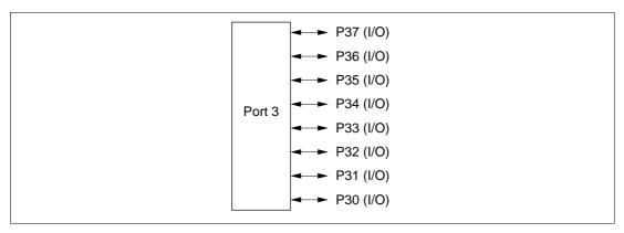
Figure 8.11 Port 3 Pin Functions (Modes 2 and 3 (EXPE = 0))
