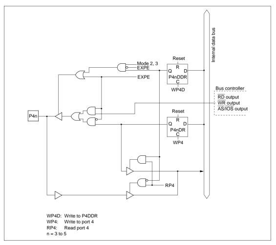
Figure C.12 Port 4 Block Diagram (Pins P43 to P45)
