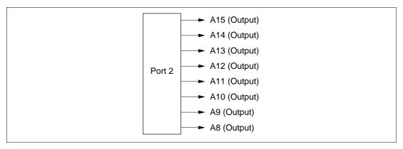
Figure 8.6 Port 2 Pin Functions (Mode 1)
