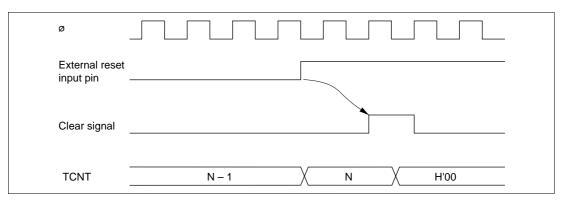
Figure 12.7 Timing of Clearing by External Reset Input
