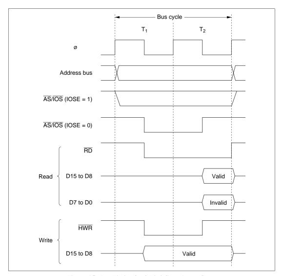
Figure 6.5 Bus Timing for 8-Bit 2-State Access Space
