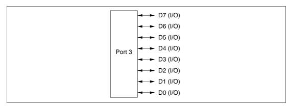
Figure 8.10 Port 3 Pin Functions (Modes 1, 2, and 3 (EXPE = 1))
