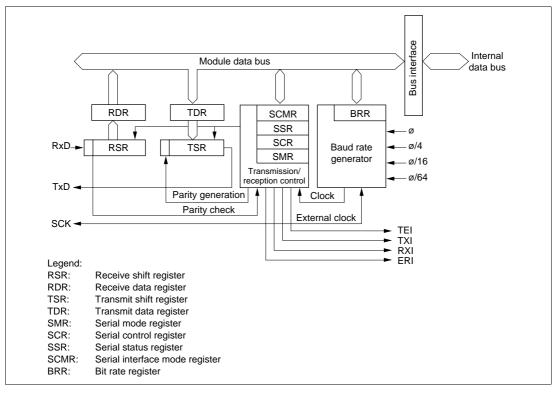
Figure 15.1 Block Diagram of SCI
