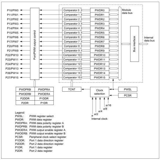
Figure 9.1 Block Diagram of PWM Timer Module
