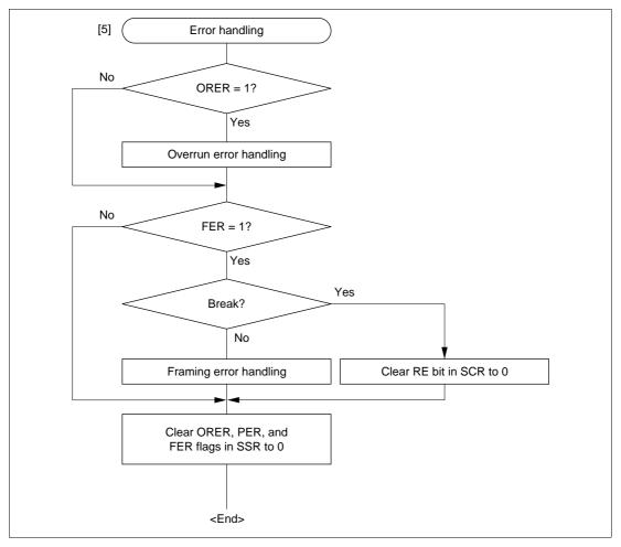
Figure 15.12 Sample Multiprocessor Serial Reception Flowchart (cont)
