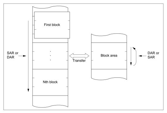
Figure 7.8 Memory Mapping in Block Transfer Mode
