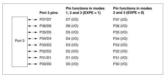
Figure 8.9 Port 3 Pin Functions
