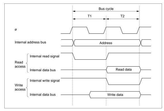
Figure 2.19 On-Chip Supporting Module Access Cycle
