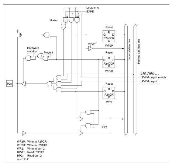
Figure C.3 Port 2 Block Diagram (Pins P20 to P22)
