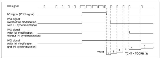
Figure 13.7 Fall Modification/IHI Synchronization Timing Chart
