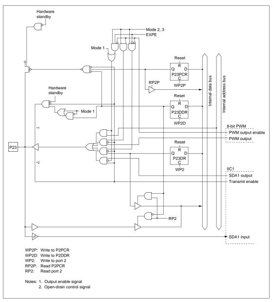
Figure C.4 Port 2 Block Diagram (Pin 23)
