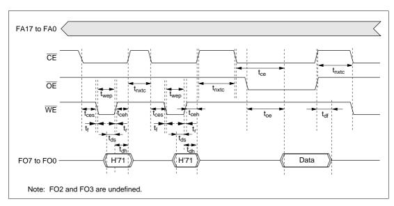
Figure 19.22 Status Read Mode Timing Waveforms
