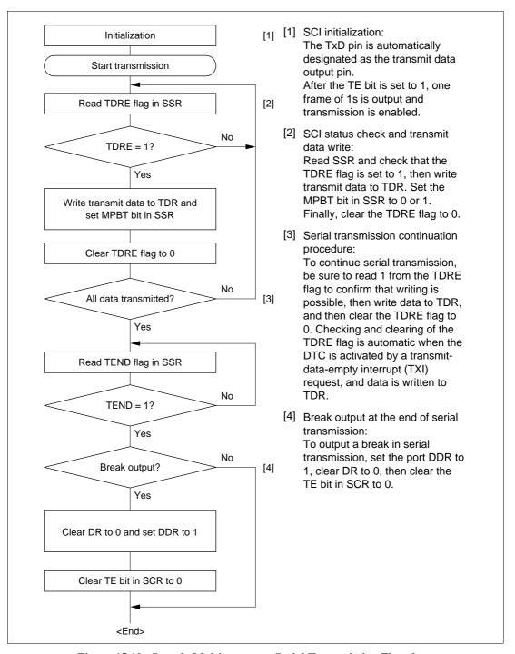
Figure 15.10 Sample Multiprocessor Serial Transmission Flowchart
