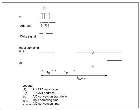
Figure 17.5 A/D Conversion Timing
