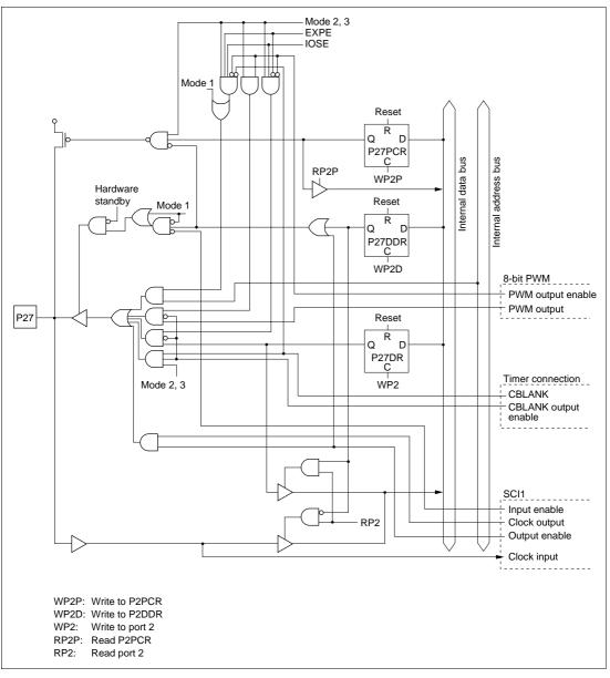
Figure C.8 Port 2 Block Diagram (Pin P27)
