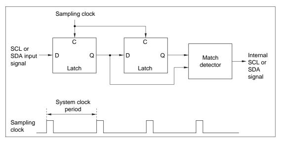
Figure 16.13 Block Diagram of Noise Canceler
