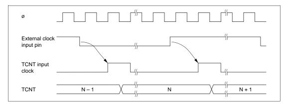
Figure 12.3 Count Timing for External Clock Input
