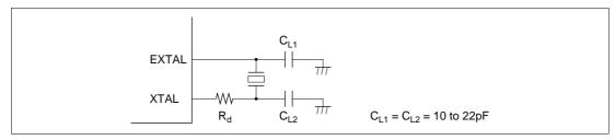
Figure 20.2 Connection of Crystal Resonator (Example)
