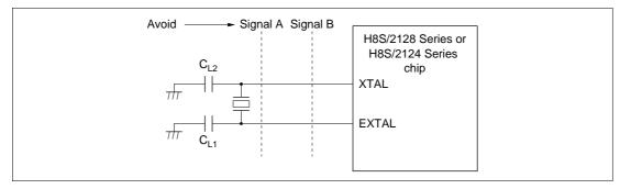
Figure 20.4 Example of Incorrect Board Design
