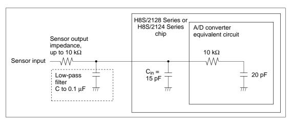
Figure 17.11 Example of Analog Input Circuit
