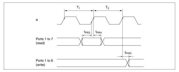
Figure 22.14 I/O Port Input/Output Timing
