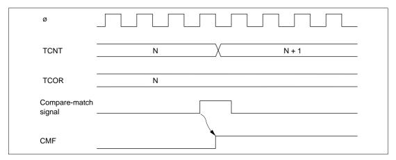
Figure 12.4 Timing of CMF Setting
