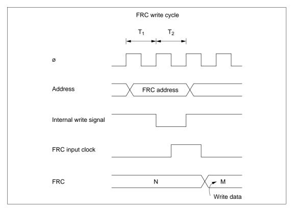
Figure 11.19 FRC Write-Increment Contention
