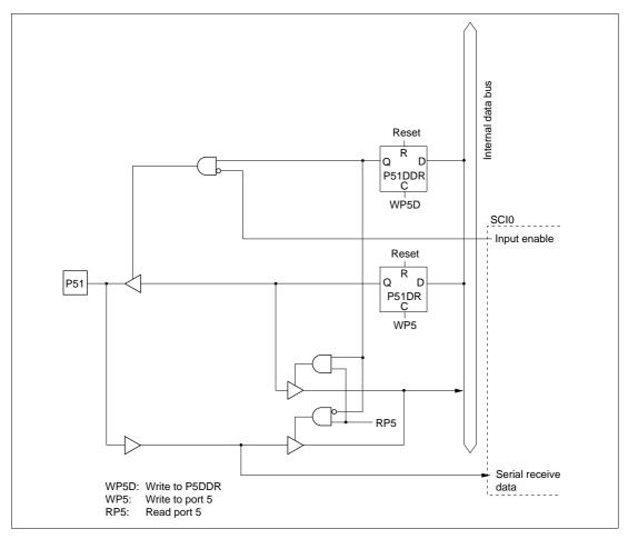
Figure C.16 Port 5 Block Diagram (Pin P51)
