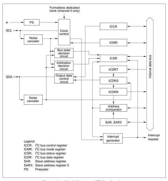
Figure 16.1 Block Diagram of  $I^2C$  Bus Interface
