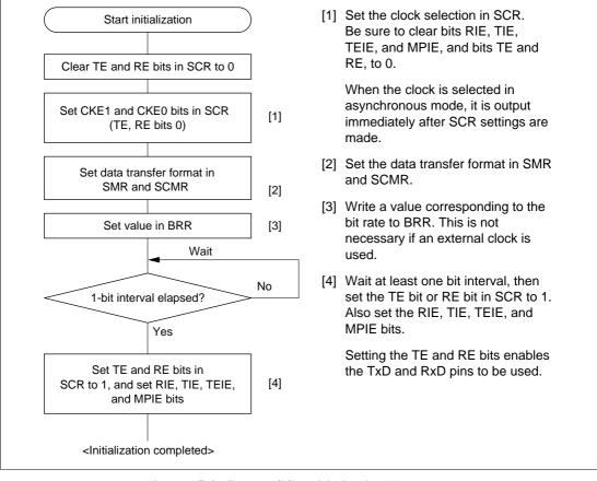
Figure 15.4 Sample SCI Initialization Flowchart
