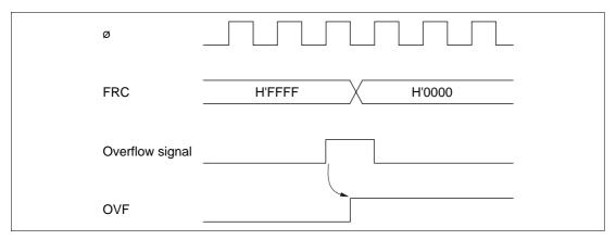
Figure 11.13 Setting of Overflow Flag (OVF)
