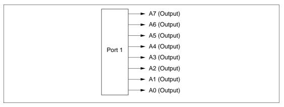
Figure 8.2 Port 1 Pin Functions (Mode 1)
