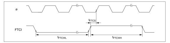
Figure 22.16 FRT Clock Input Timing
