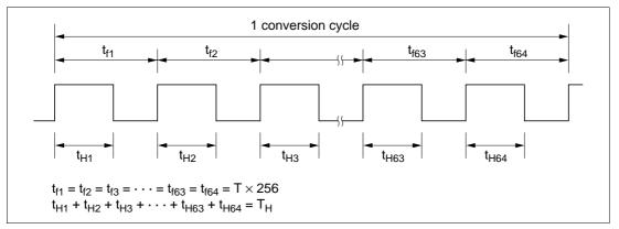
Figure 10.4 (4) Output Waveform
