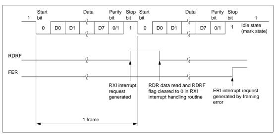
Figure 15.8 Example of SCI Operation in Reception (Example with 8-Bit Data, Parity, One Stop Bit)
