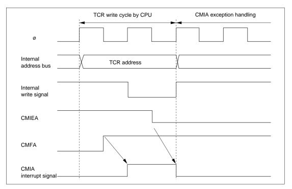
Figure 5.11 Contention between Interrupt Generation and Disabling
