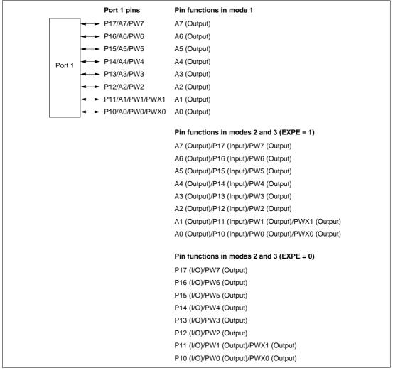
Figure 8.1 Port 1 Pin Functions
