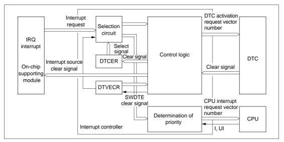
Figure 5.12 Interrupt Control for DTC
