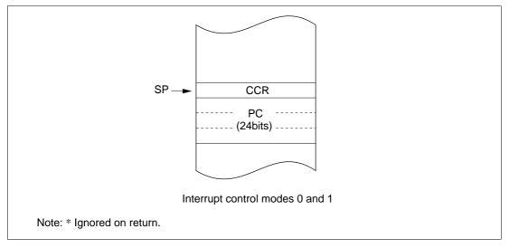
Figure 4.5 (2) Stack Status after Exception Handling (Advanced Mode)
