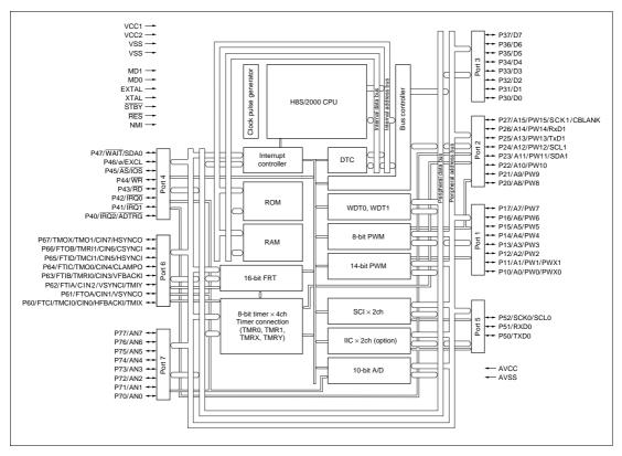
Figure 1.1 Internal Block Diagram of H8S/2128 Series
