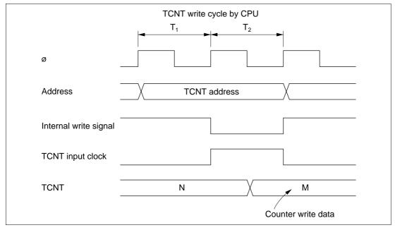
Figure 12.11 Contention between TCNT Write and Increment
