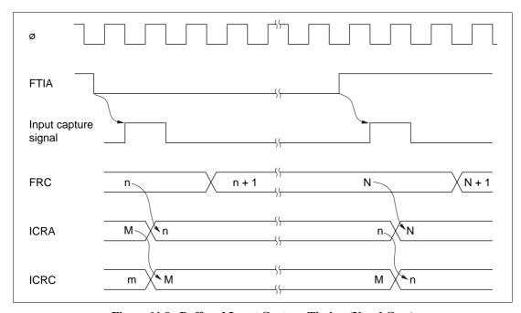
Figure 11.9 Buffered Input Capture Timing (Usual Case)
