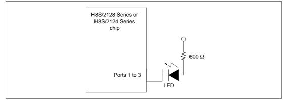
Figure 22.2 LED Drive Circuit (Example)
