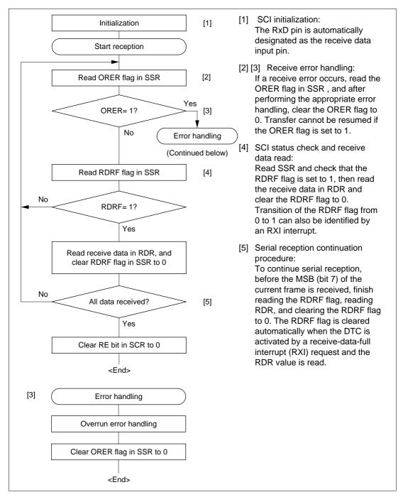
Figure 15.18 Sample Serial Reception Flowchart
