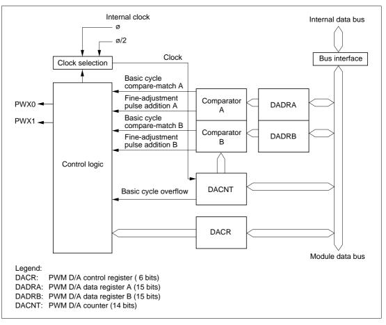
Figure 10.1 PWM D/A Block Diagram
