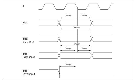
Figure 22.8 Interrupt Input Timing
