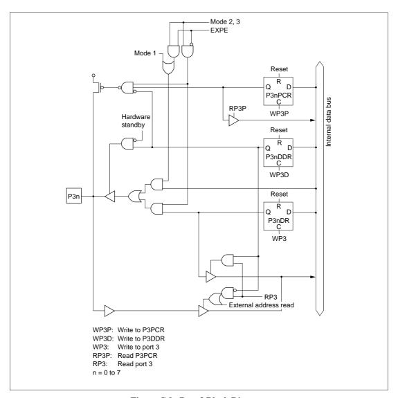
Figure C.9 Port 3 Block Diagram
