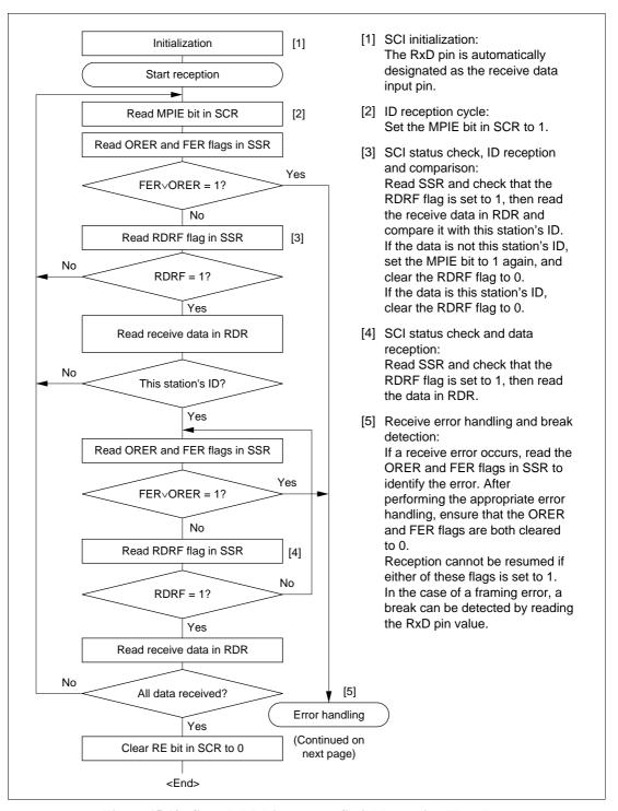
Figure 15.12 Sample Multiprocessor Serial Reception Flowchart
