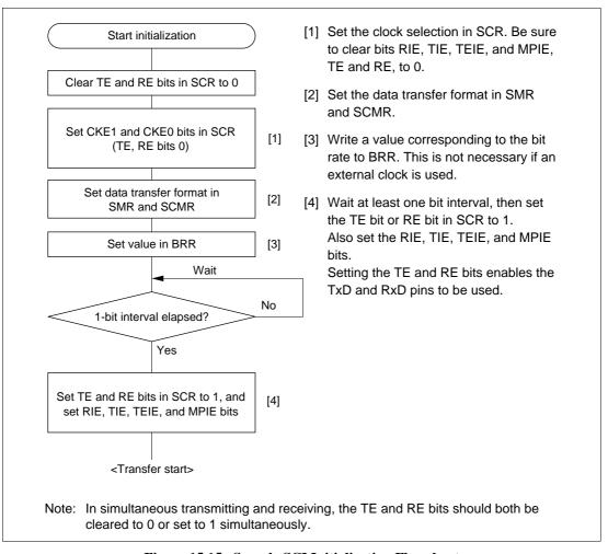
Figure 15.15 Sample SCI Initialization Flowchart
