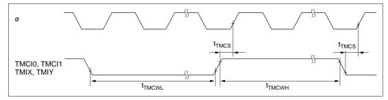
Figure 22.18 8-Bit Timer Clock Input Timing
