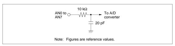
Figure 17.8 Analog Input Pin Equivalent Circuit
