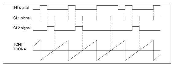
Figure 13.3 Timing Chart for Clamp Waveform Generation (CL1 and CL2 Signals)
