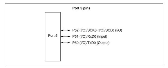
Figure 8.13 Port 5 Pin Functions
