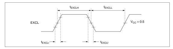
Figure 20.8 Subclock Input Timing
