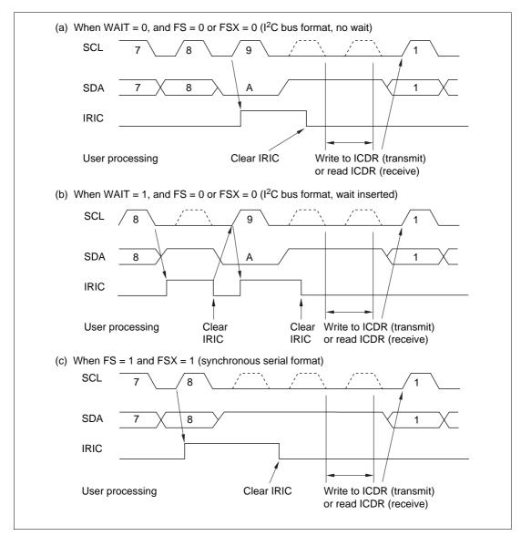
Figure 16.12 IRIC Setting Timing and SCL Control
