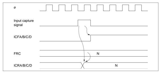
Figure 11.11 Setting of Input Capture Flag (ICFA/B/C/D)
