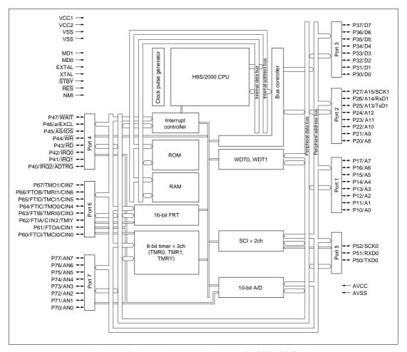
Figure 1.2 Internal Block Diagram of H8S/2124 Series
