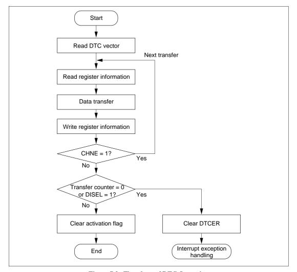
Figure 7.2 Flowchart of DTC Operation
