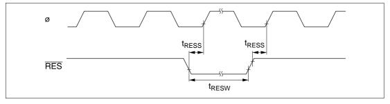
Figure 22.7 Reset Input Timing
