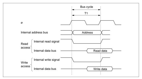
Figure 2.17 On-Chip Memory Access Cycle
