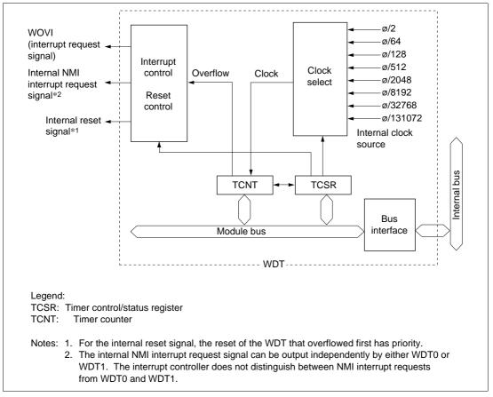
Figure 14.1 (a) Block Diagram of WDT0
