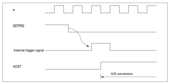
Figure 17.6 External Trigger Input Timing
