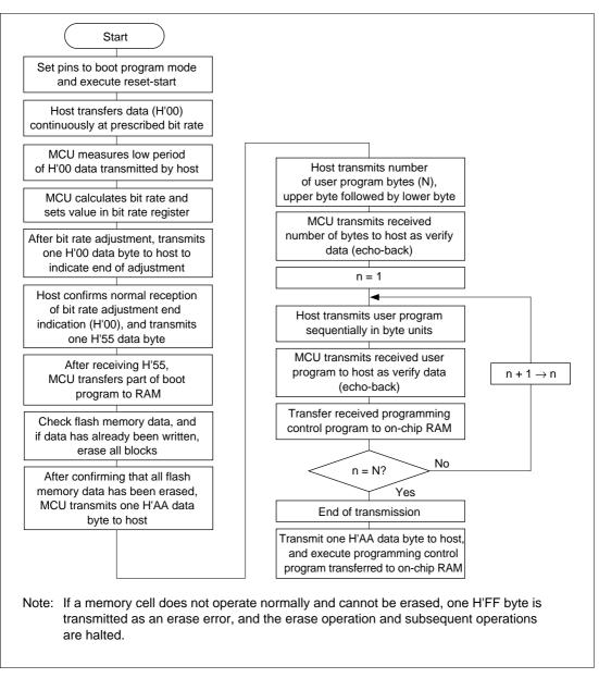
**Figure 19.8 Boot Mode Execution Procedure**
