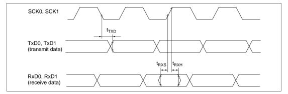
Figure 22.22 SCI Input/Output Timing (Synchronous Mode)
