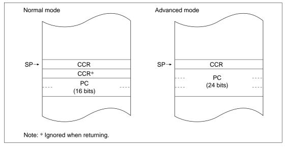
Figure 2.16 Stack Structure after Exception Handling (Examples)
