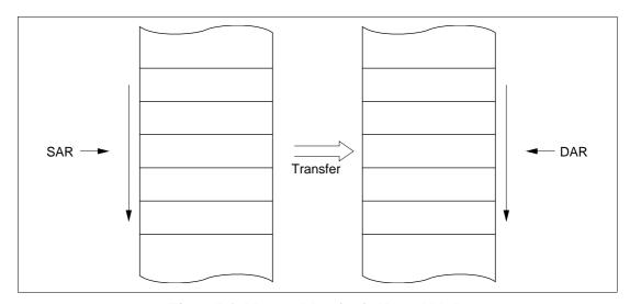
Figure 7.6 Memory Mapping in Normal Mode
