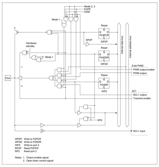
Figure C.5 Port 2 Block Diagram (Pin 24)
