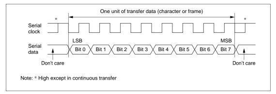
Figure 15.14 Data Format in Synchronous Communication
