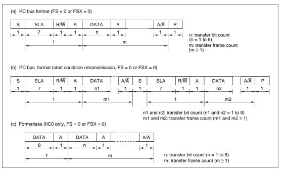
Figure 16.3 I<sup>2</sup>C Bus Data Formats (I<sup>2</sup>C Bus Formats)
