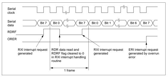
Figure 15.19 Example of SCI Operation in Reception
