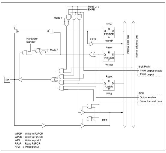
Figure C.6 Port 2 Block Diagram (Pin P25)
