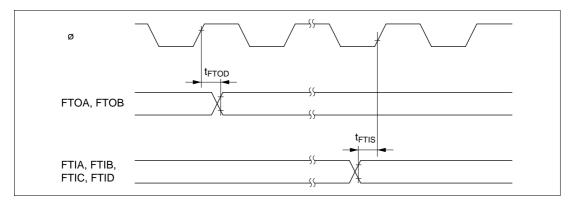
Figure 22.15 FRT Input/Output Timing
