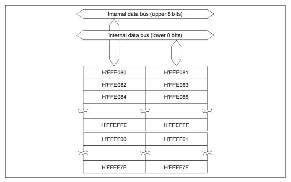
Figure 18.1 Block Diagram of RAM (H8S/2128, H8S/2124, H8S/2123)
