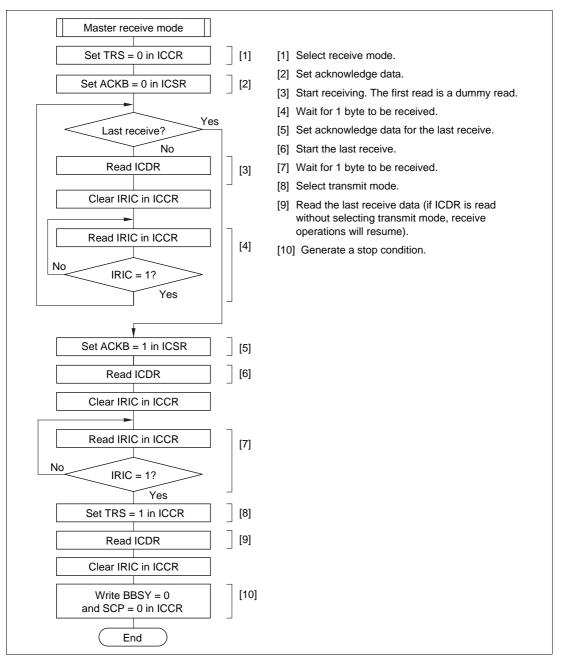
Figure 16.15 Flowchart for Master Receive Mode (Example)
