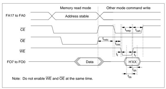
Figure 19.17 Timing Waveforms when Entering Another Mode from Memory Read Mode
