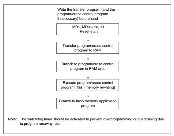
Figure 19.11 User Program Mode Execution Procedure
