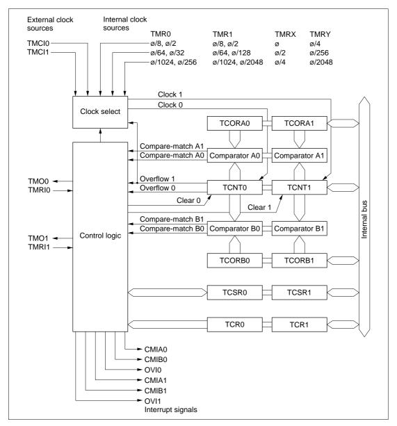
Figure 12.1 Block Diagram of 8-Bit Timer Module
