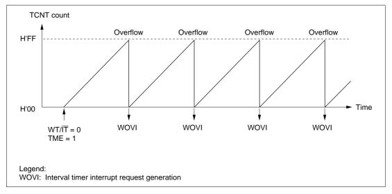
Figure 14.4 Operation in Interval Timer Mode
