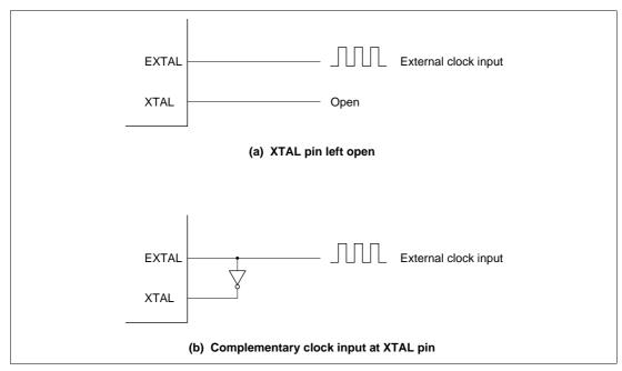
Figure 20.5 External Clock Input (Examples)
