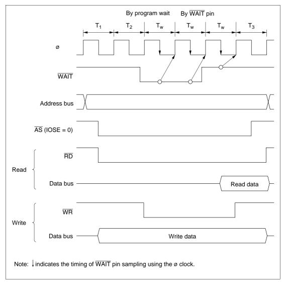
Figure 6.7 Example of Wait State Insertion Timing
