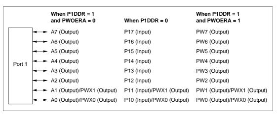
Figure 8.3 Port 1 Pin Functions (Modes 2 and 3 (EXPE = 1))
