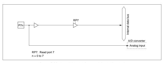
Figure C.23 Port 7 Block Diagram (Pins P70 to P77)
