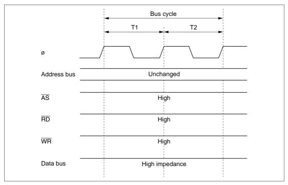
Figure 2.20 Pin States during On-Chip Supporting Module Access
