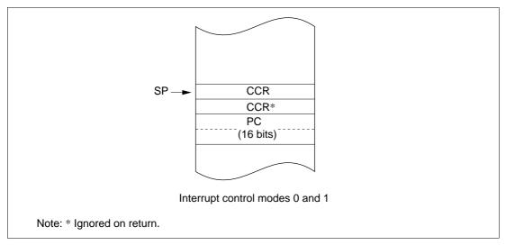
Figure 4.5 (1) Stack Status after Exception Handling (Normal Mode)
