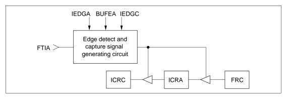
Figure 11.2 Input Capture Buffering (Example)
