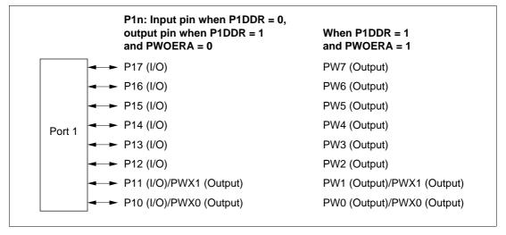
Figure 8.4 Port 1 Pin Functions (Modes 2 and 3 (EXPE = 0))
