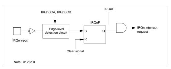
Figure 5.2 Block Diagram of Interrupts IRQ2 to IRQ0
