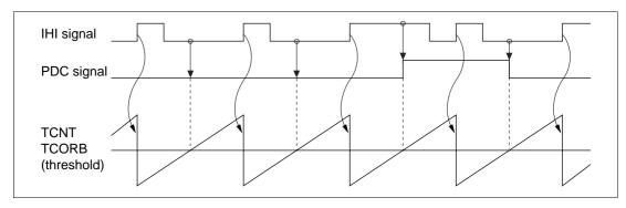
Figure 13.2 Timing Chart for PWM Decoding
