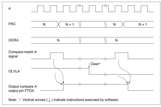
Figure 11.5 Timing of Output Compare A Output
