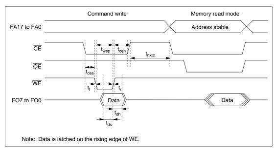
Figure 19.16 Memory Read Mode Timing Waveforms after Command Write
