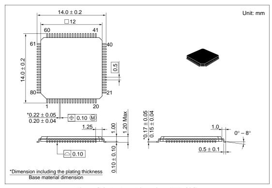
Figure G.3 Package Dimensions (TFP-80C)
