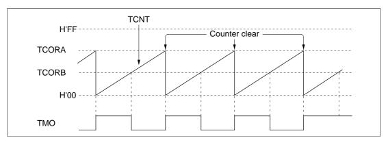
Figure 12.9 Pulse Output (Example)
