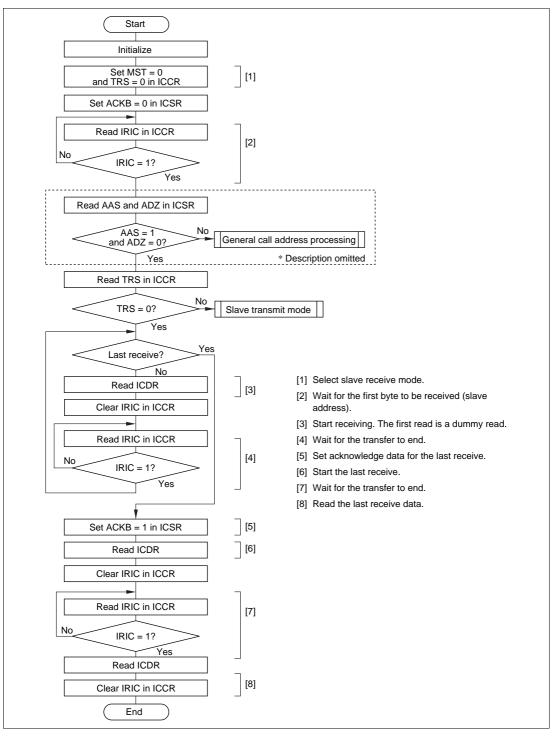
Figure 16.16 Flowchart for Slave Receive Mode (Example)
