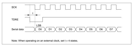
Figure 15.22 Example of Synchronous Transmission by DTC
