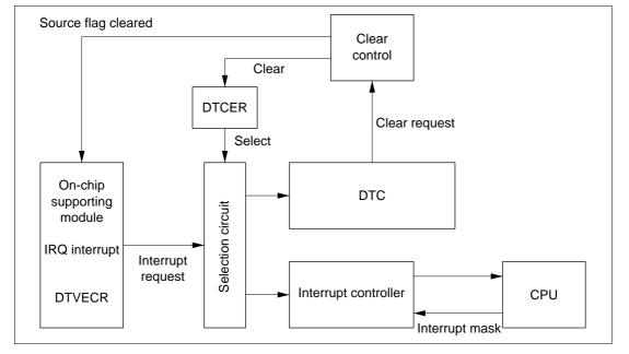
Figure 7.3 Block Diagram of DTC Activation Source Control
